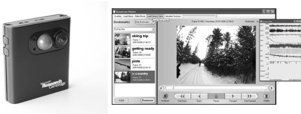
Figure 4. (left) SenseCam and (right) the interface used to review images. Salient moments can be flagged with bookmarks, and the images can be reviewed at various speeds.
