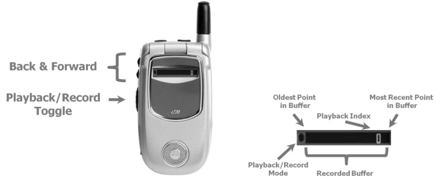
Figure 3. (left) Personal Audio Loop system in its prototype form used for pilot deployment study. (right) The review interface is largely audio-based, but there are some visual elements to help users recognize their mode and where they are in the audio buffer when playing back sound.
